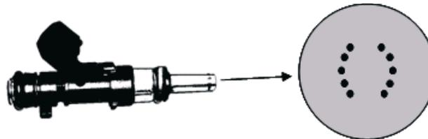
Fig. 2. Drawing of injector holes configuration
