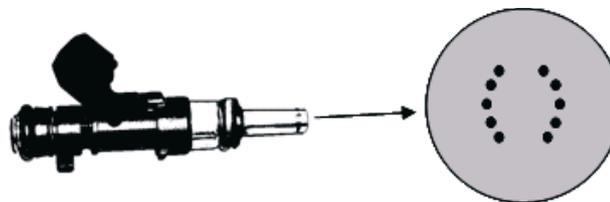
Fig. 2. Drawing of injector holes configuration
